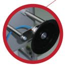
Holding to the panel using a suction vacuum pump, which can be positioned horizontally or vertically
