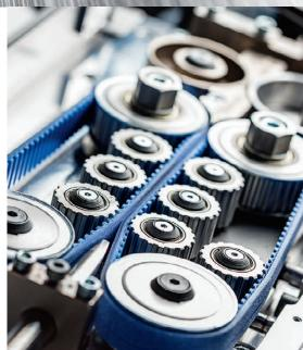
The efficient belt drive reliably draws in the cable at a speed of up to 9 m/s.
