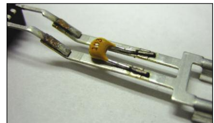
Capacitor to lead frame
