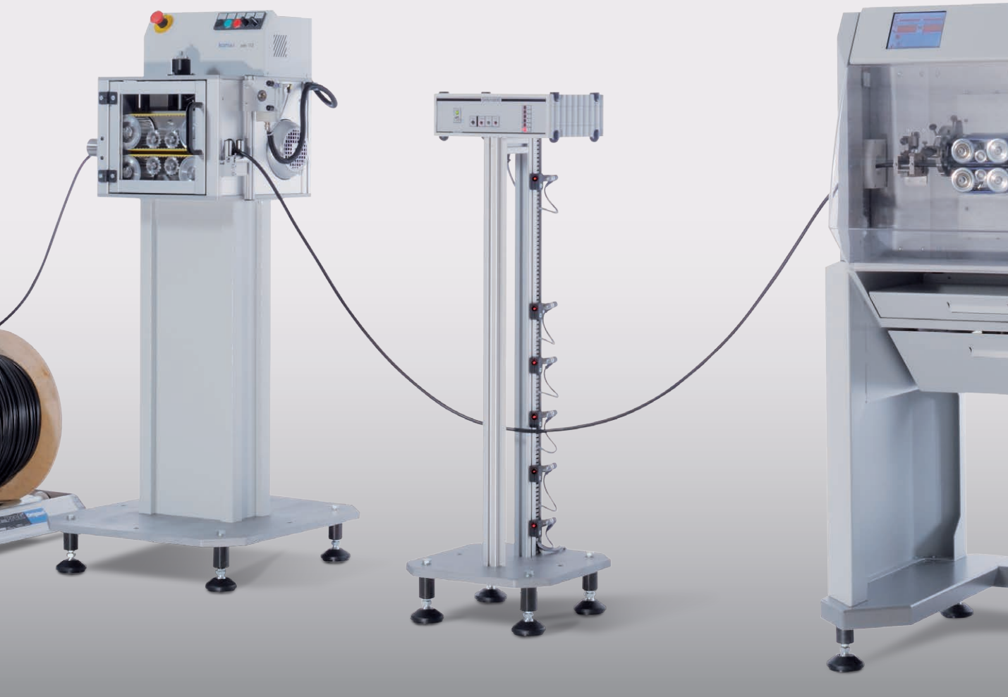
▲ ads 112 Wire pull machine with DHS 1000D wire sage control unit on a Kappa 350
