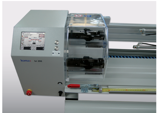
▲ bt 288 Intuitive TopTouch control system and two twisting lines
