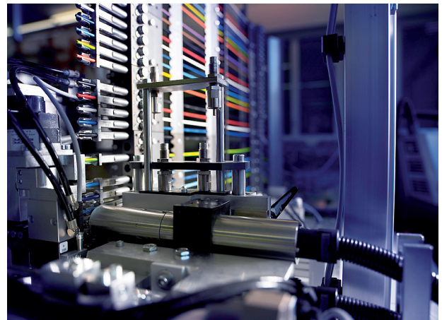
▲ Automatic marking head changer on Zeta Cable replacement without operator intervention, thanks to automatic text centering
