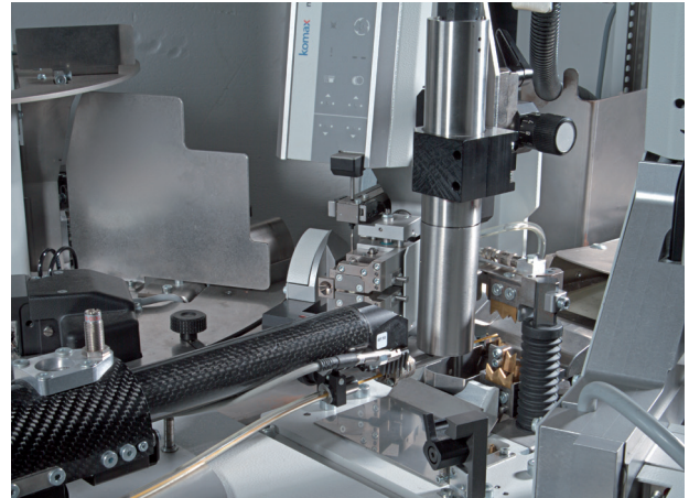
▲ ims 295 on Alpha 455 Minimal zero-cut, as the print head is positioned close to the cutting head
