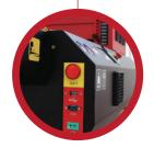
Side panel with USB port for reference uploading and barcode reader connection
