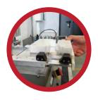
Fast removable shrinking chamber (less than 2 seconds to swap)
